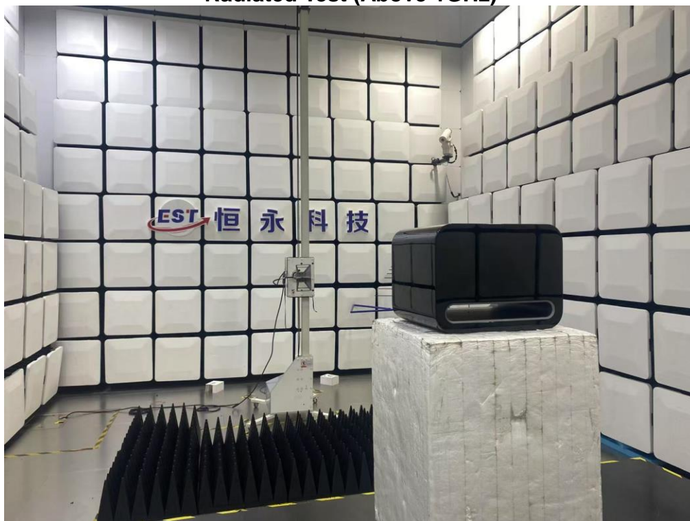
Radiated Test (Above 1GHz)
