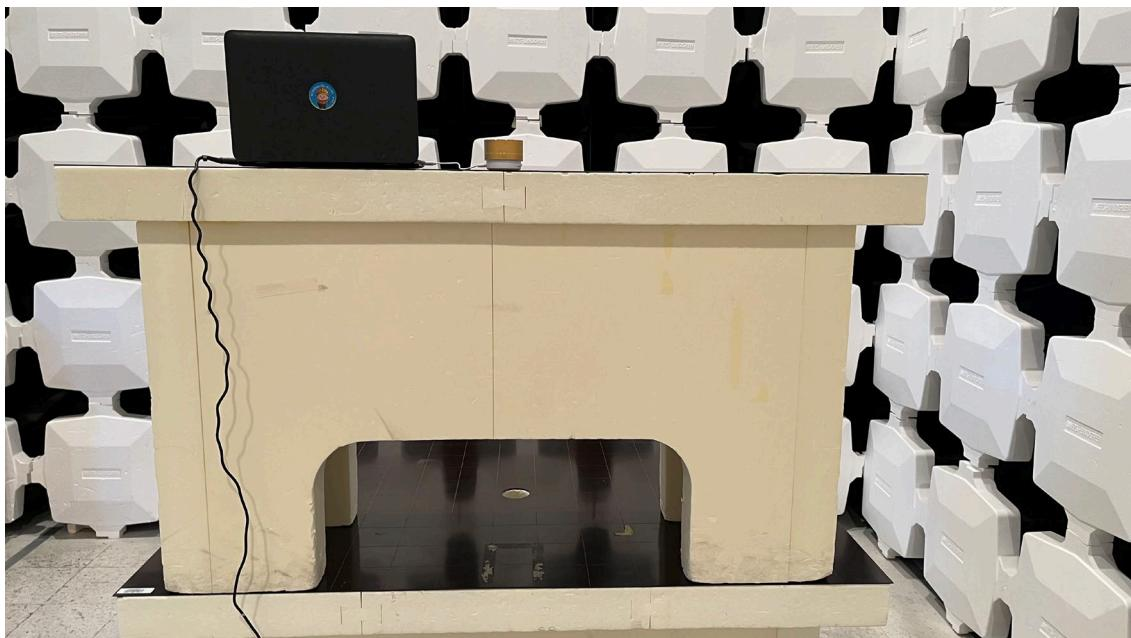
The unit was placed in the center of the turntable.
