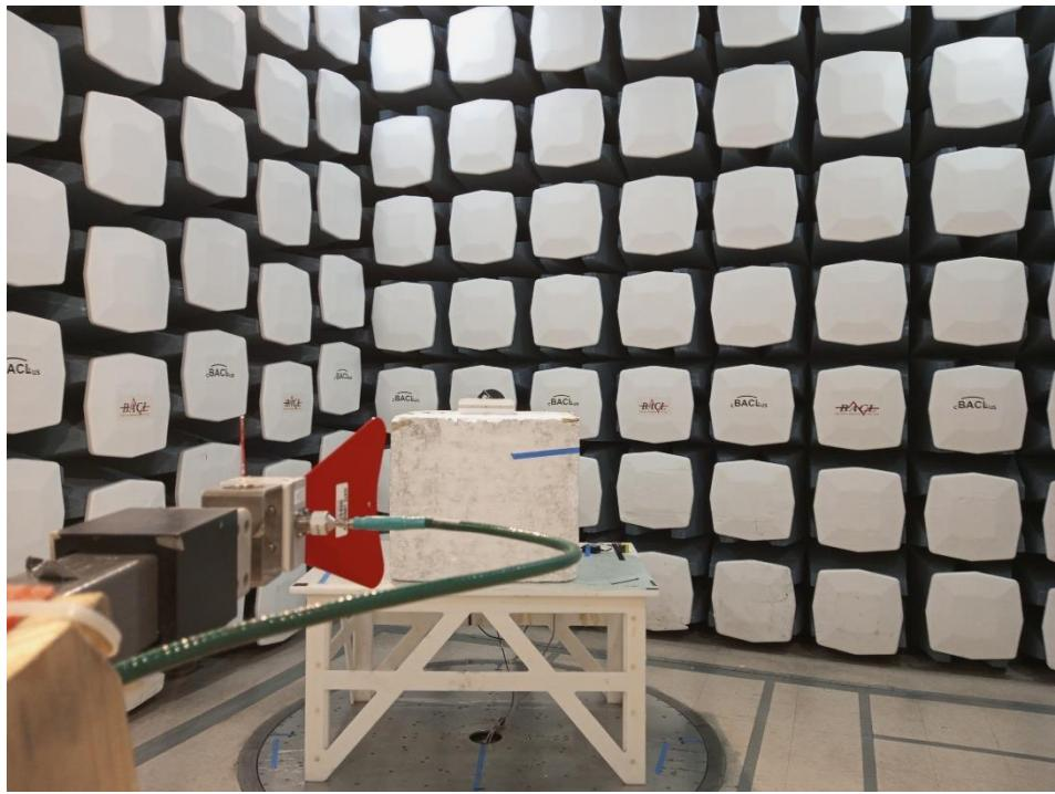
**1.6 Radiated Spurious Emissions: 1 GHz to 18 GHz, Rear View at 3 meters distance**
