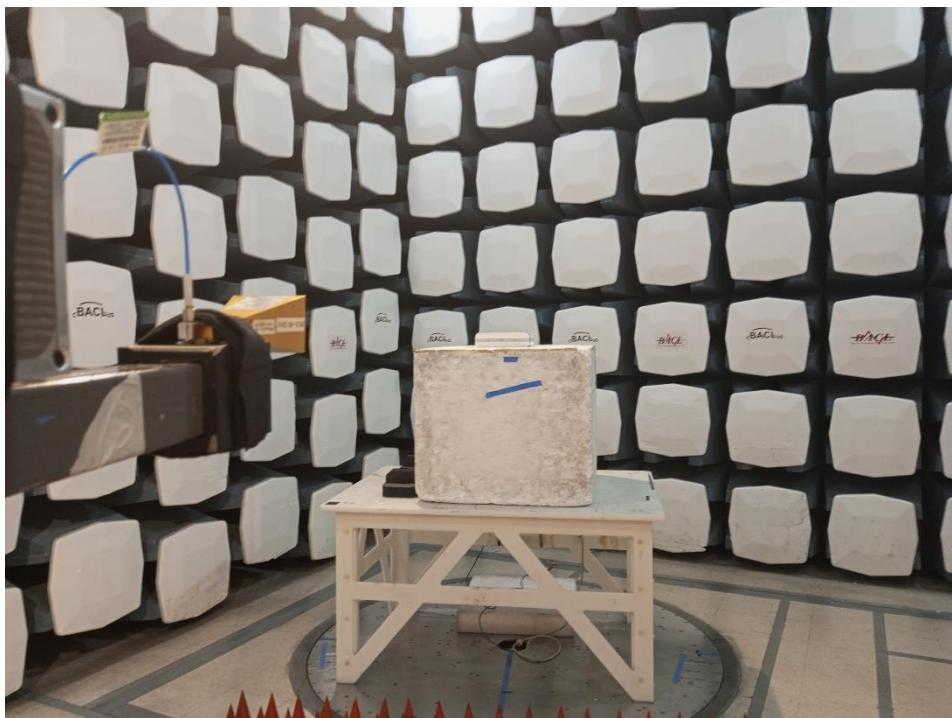
**1.10 Radiated Spurious Emissions: 26.5 GHz to 40 GHz, Rear View at 3 meters distance**
