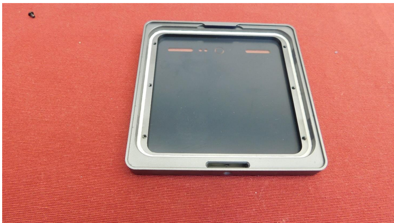
Picture 8: Housing without keyboard layout internal view
