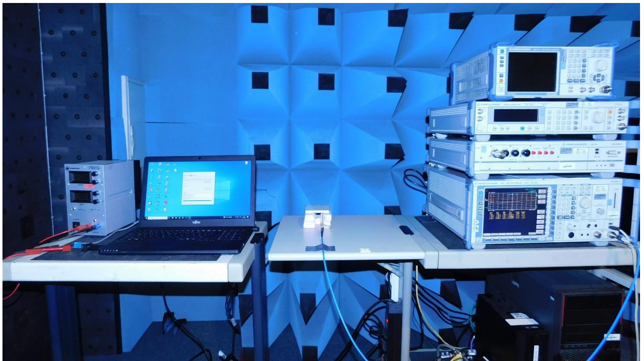
Picture 21: Antenna-port conducted spurious emissions measurements_RS-485
