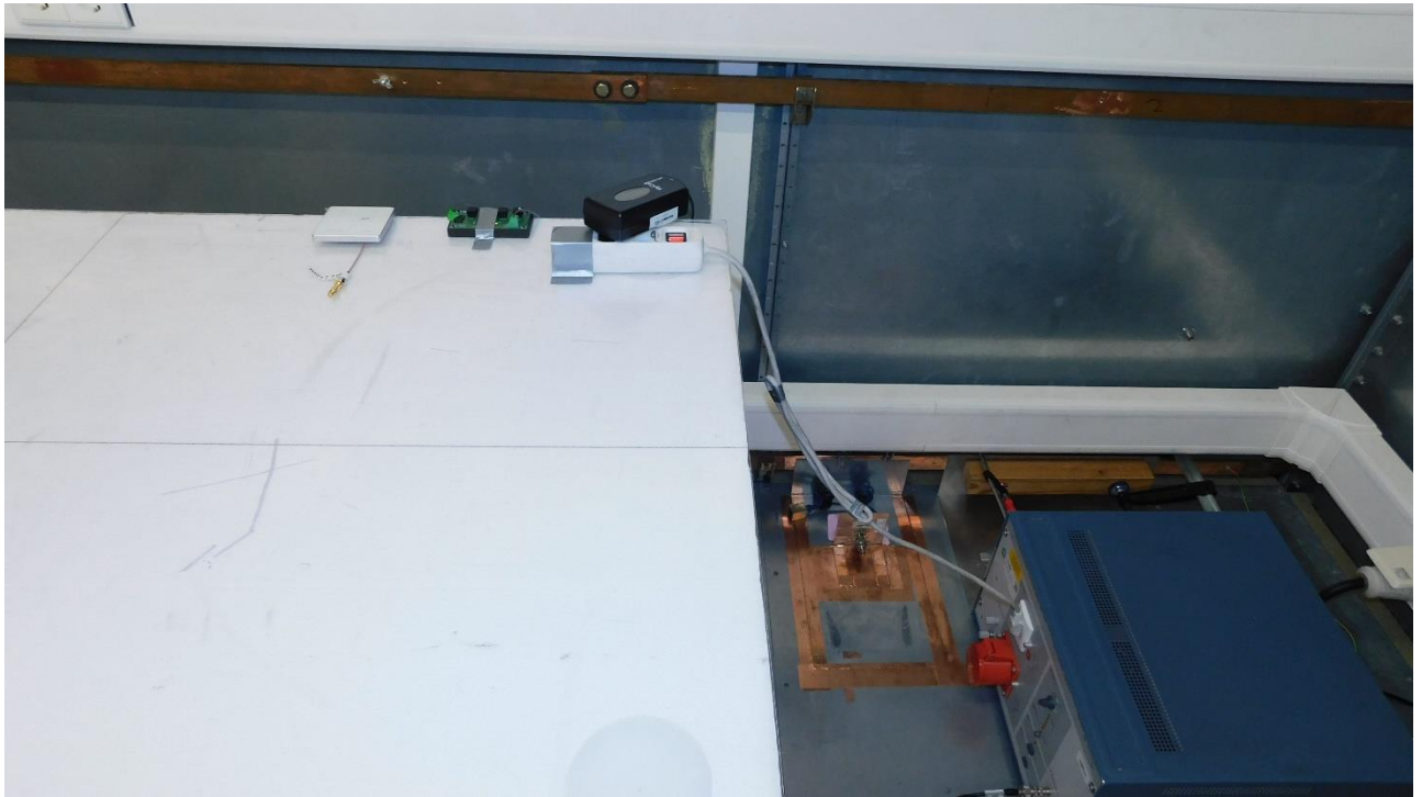
Picture 17: Test setup AC power line conducted emissions (front view)_Wiegand
