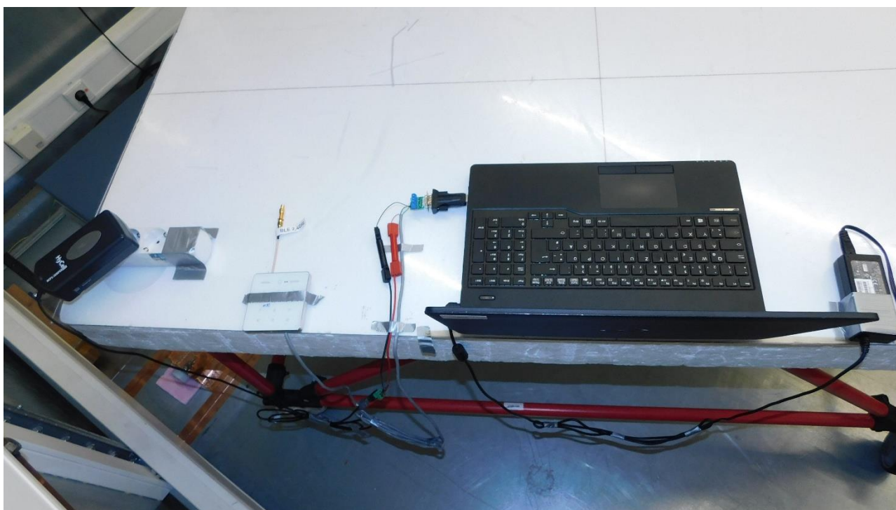
Picture 16: Test setup AC power line conducted emissions (rear view)_RS-485
