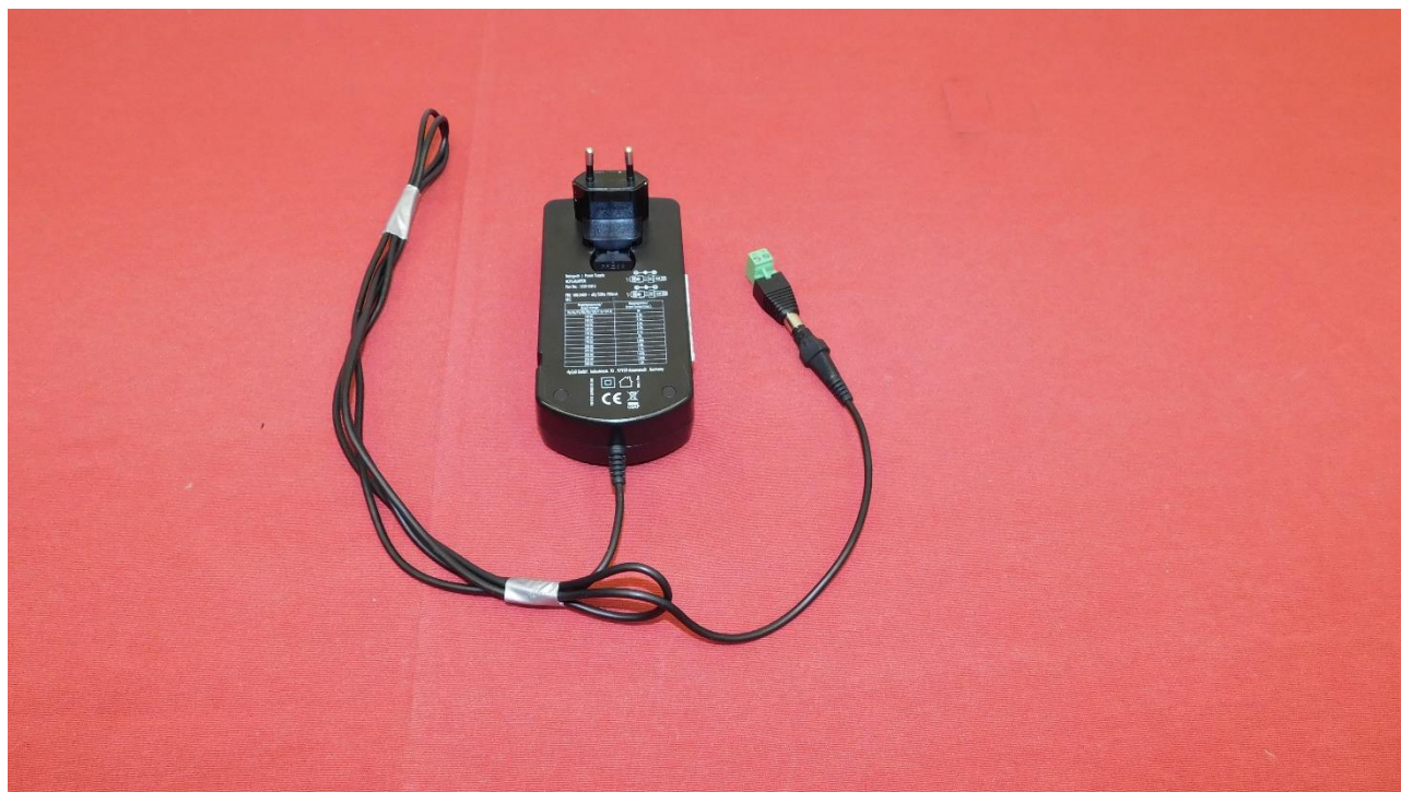
Picture 17: Power adapter used for AC power line conducted emissions measurement
