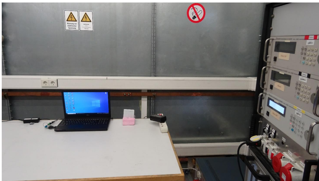
Picture 13: Test setup AC power line conducted emissions (front view)_RS-485
