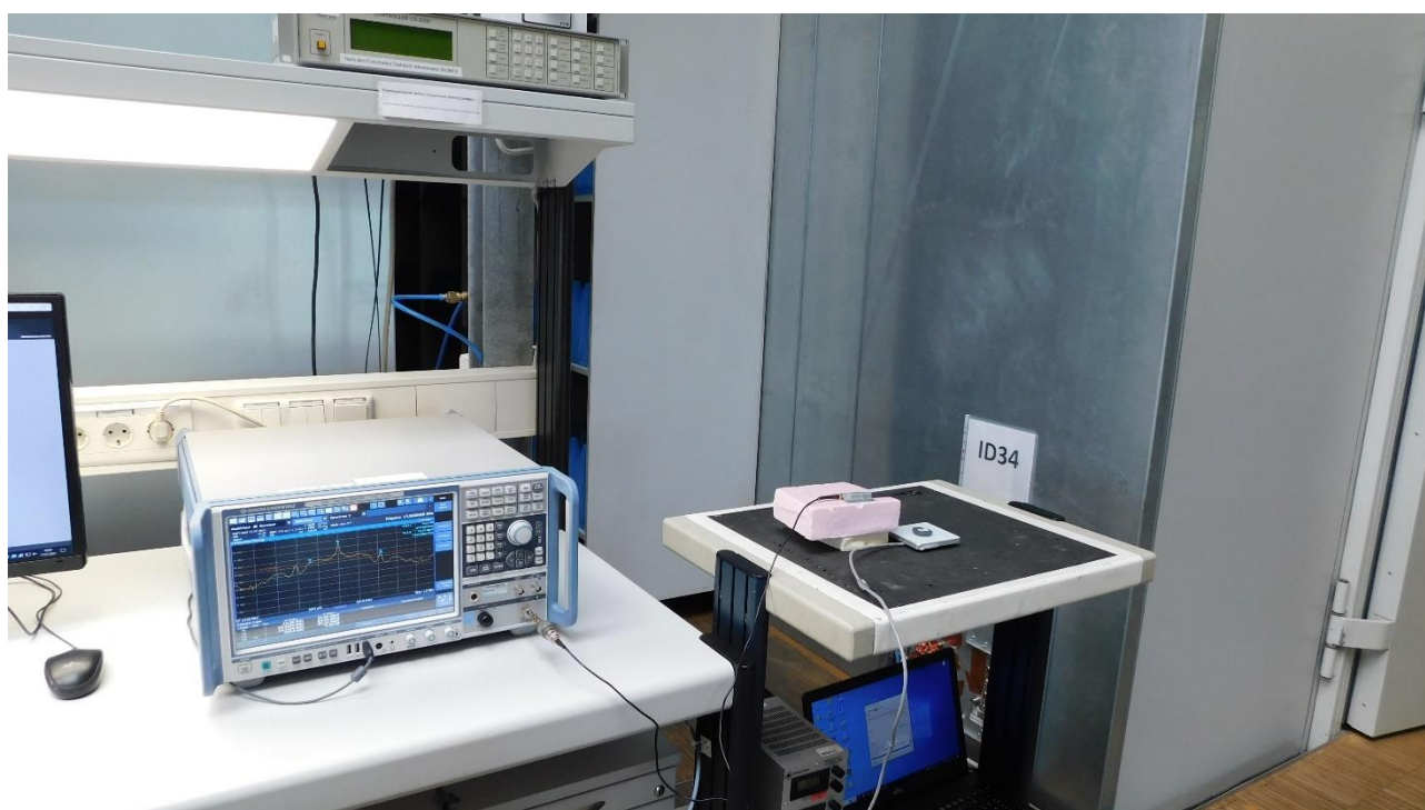
Picture 18: Bandwidth measurements_RS-485
