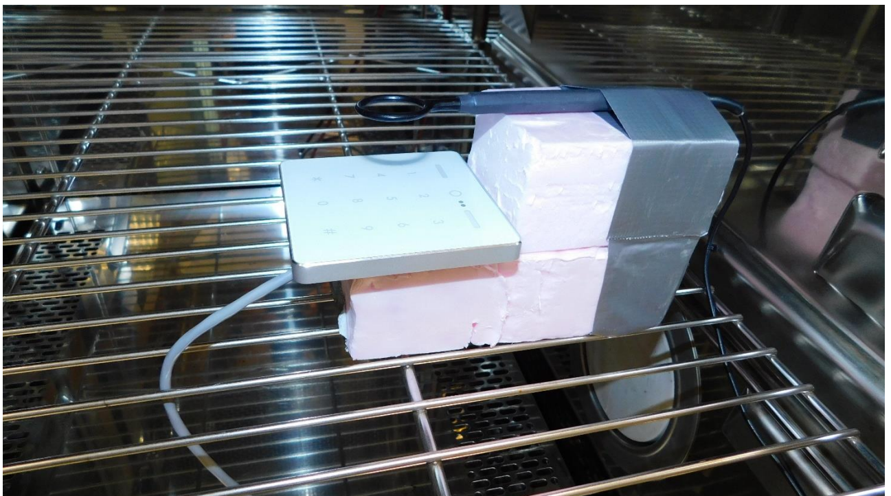
Picture 20: Carrier frequency stability test in climate chamber_RS-485 and Wiegand
