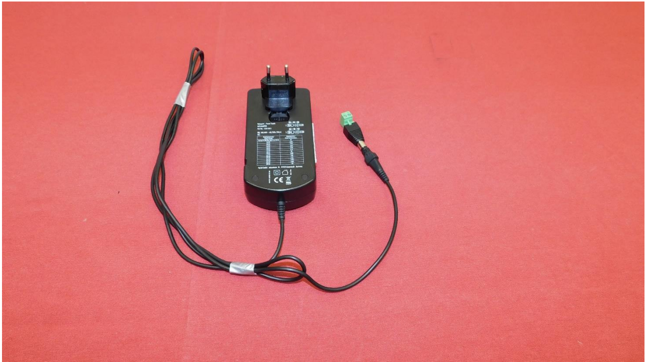
Picture 17: Power adapter used for AC power line conducted emissions measurement
