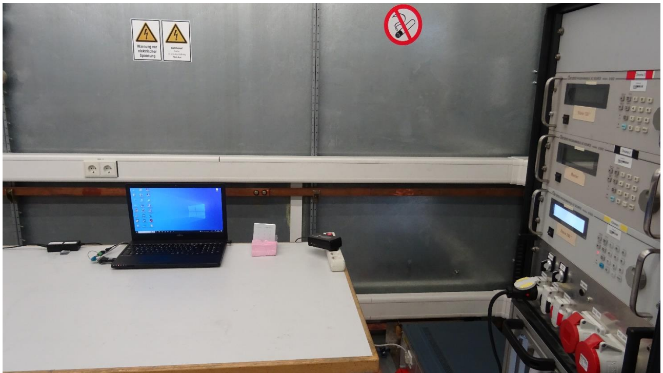
Picture 13: Test setup AC power line conducted emissions (front view)_RS-485
