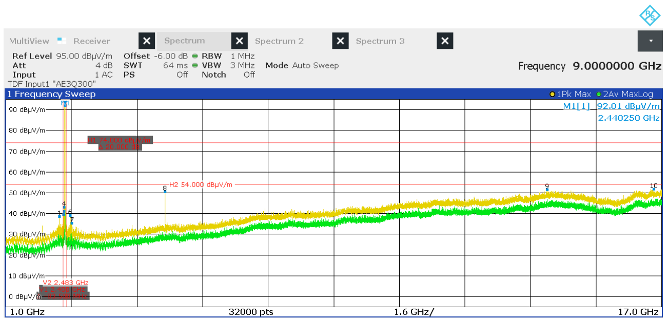
Figure 52: Chart of radiated emissions pre-measurement from 1 GHz to 17 GHz on middle channel, EUT position Y, antenna polarization horizontal
