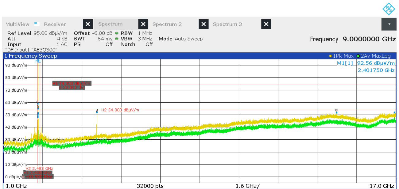
Figure 49: Chart of radiated emissions pre-measurement from 1 GHz to 17 GHz on lowest channel, EUT position Y, antenna polarization horizontal
