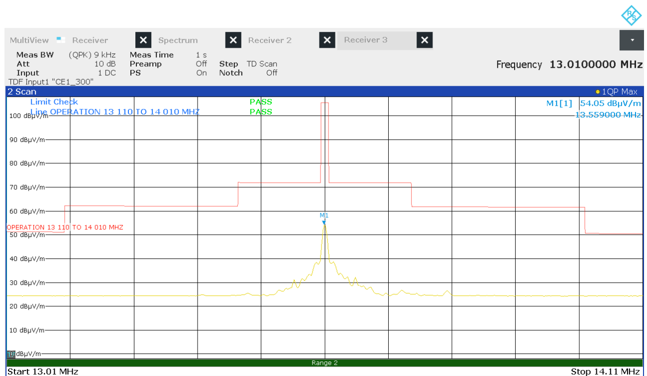
Figure 14: Chart of emission within the band 13.110 MHz to 14.010 MHz, EUT in position Z, without tag, antenna in line at 3 m distance
