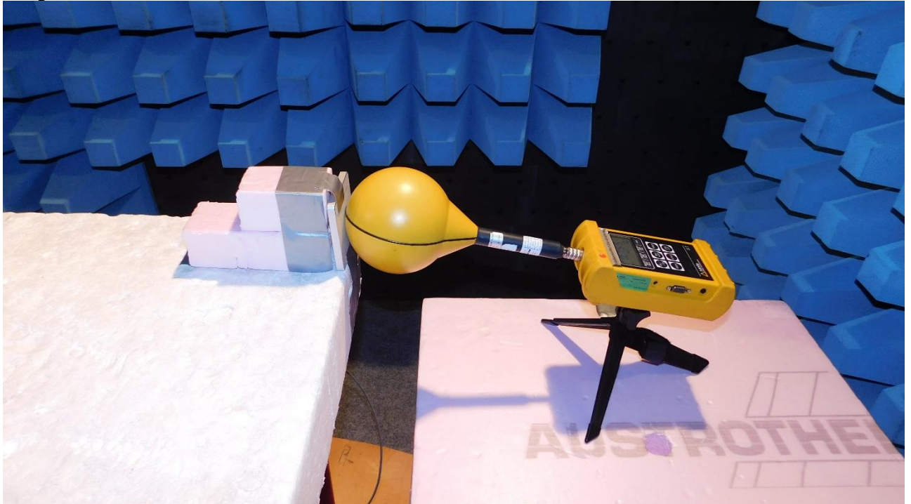
Picture 9: Setup of magnetic field test at touch position, without tag
