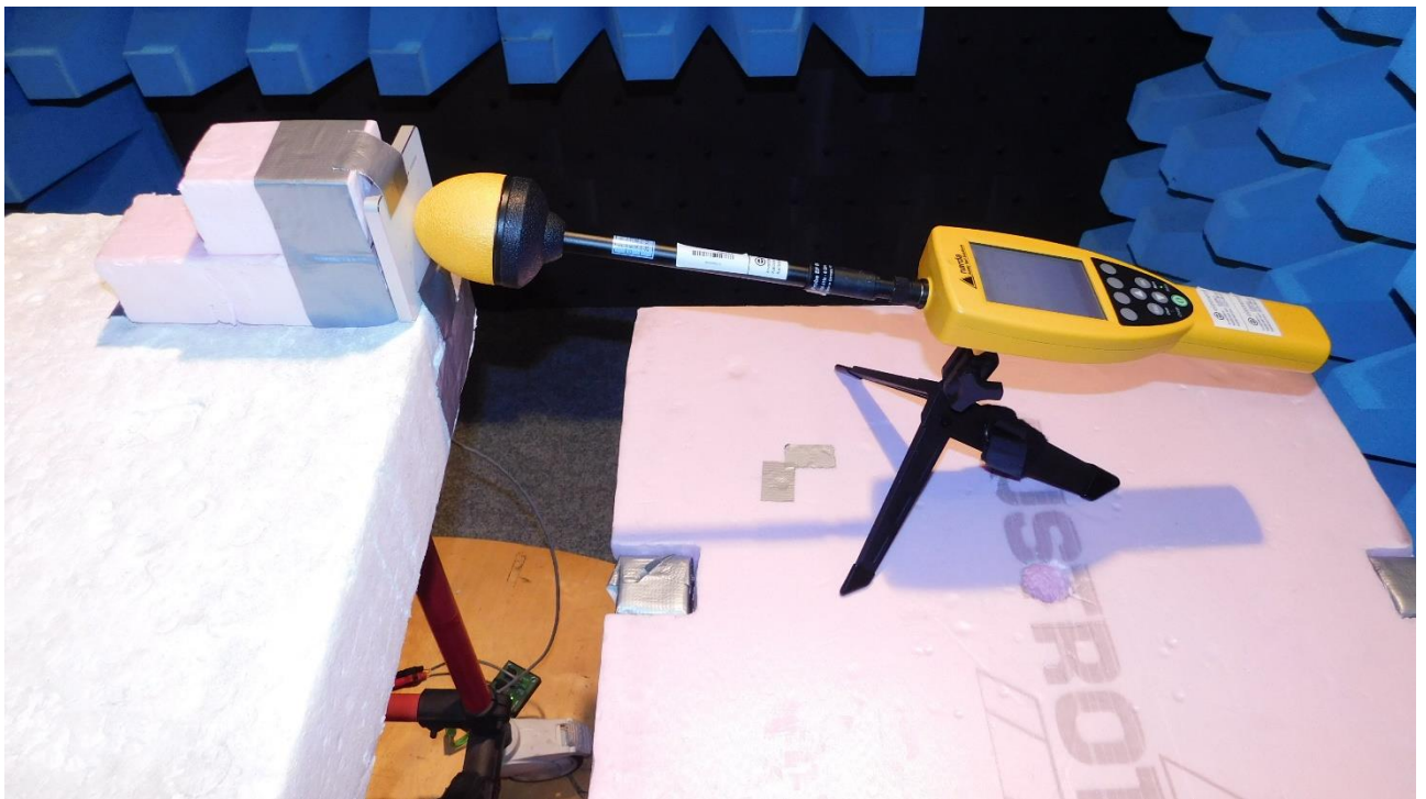
Picture 10: Setup of electric field test at touch position, without tag
