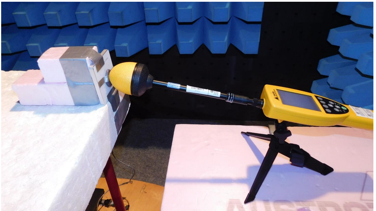
Picture 6: Setup of electric field test at touch position, with tag
