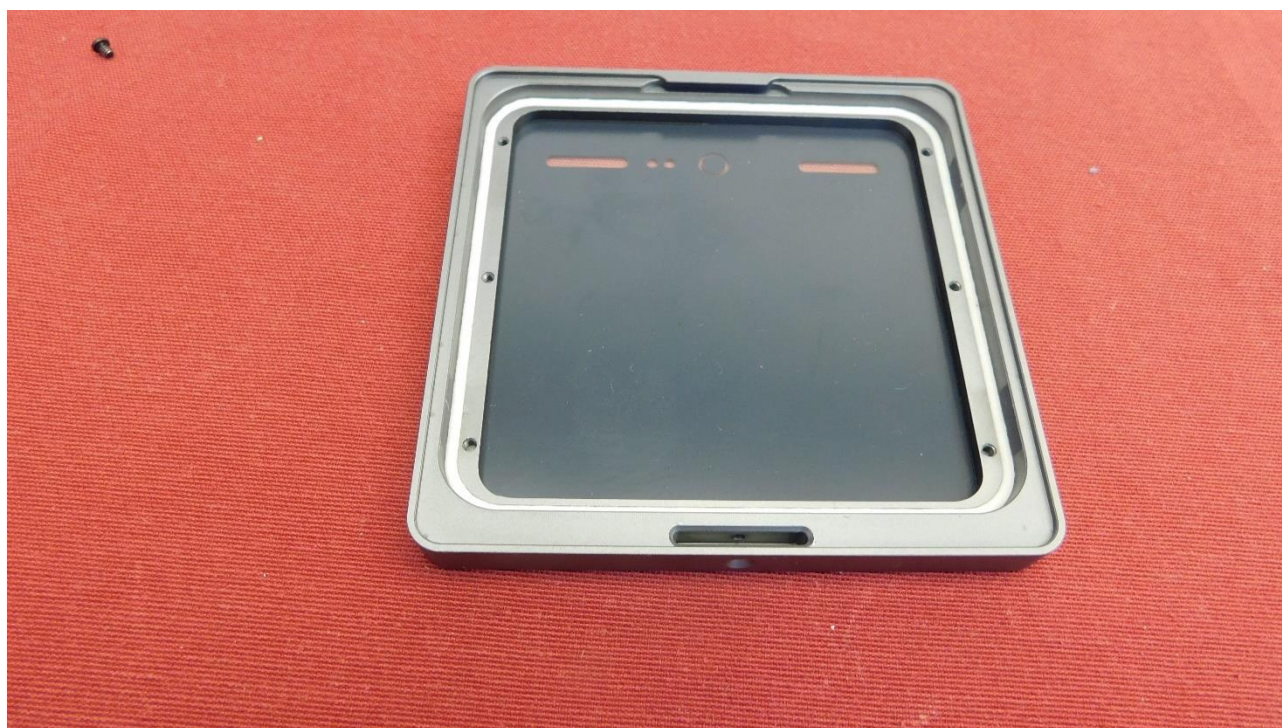
Picture 8: Housing without keyboard layout internal view
