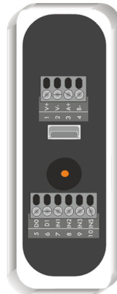
Fig. 9 - connectors on Secustos MU20 reader models
