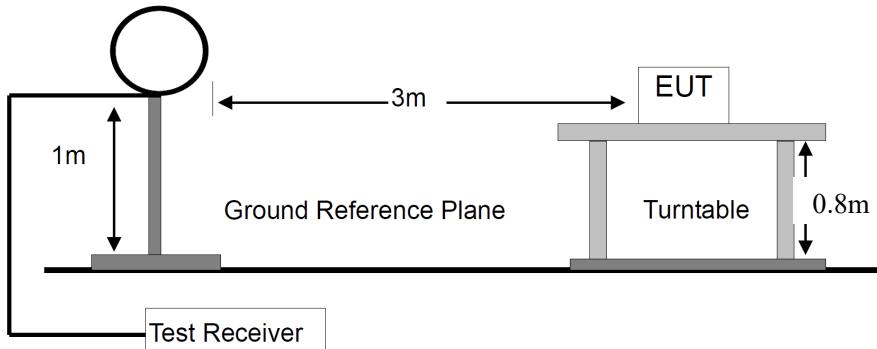
For Radiated Emission 30-1000MHz
