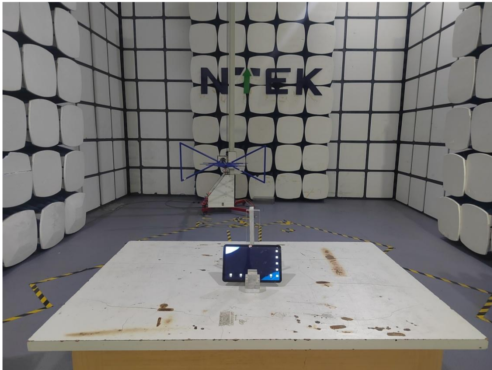
Radiated Measurement Photos(30MHz~1GHz )
