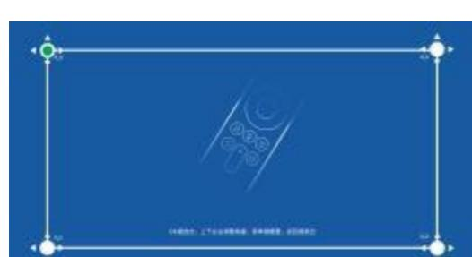
Select the four corners of image via direction button , click "OK", you can choose corresponding corner and adjust balance via direction button , press OK button and finish setting for this corner. Other corners can be adjusted like this. Press "down" button , click "OK" to enter the next step .
