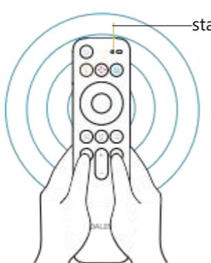
Hold the remote controller within 50cm distance from the main device, long press Home button and previous page button .
