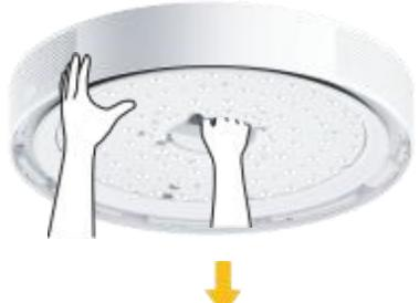
Take down the main device from the fixing bracket.
