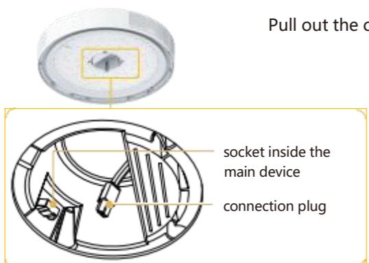
Pull out the connector plug from the socket inside the main device.
