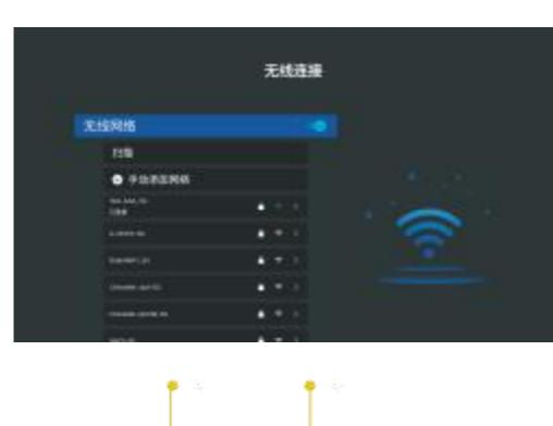
According to the network detected on the screen, press up and down button to choose the network, click "OK" to confirm.
