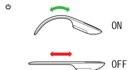
Bend the mouse to turn on power. Flatten to turn off.
