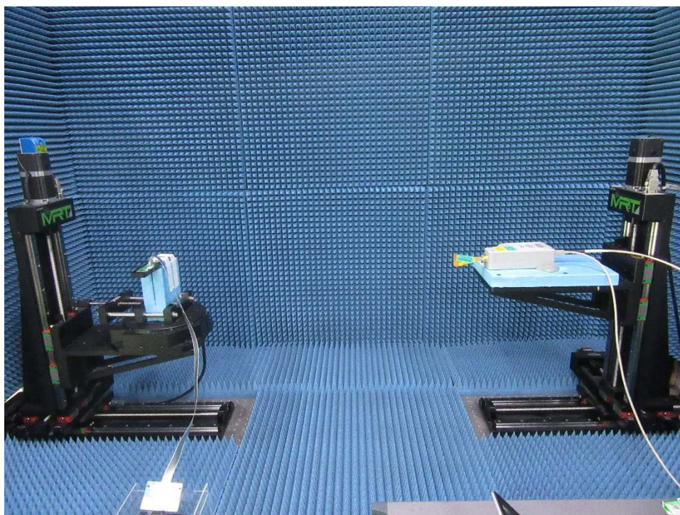
Photograph 6: Set-up photo for Radiated Spurious Emission, 75GHz - 110GHz
