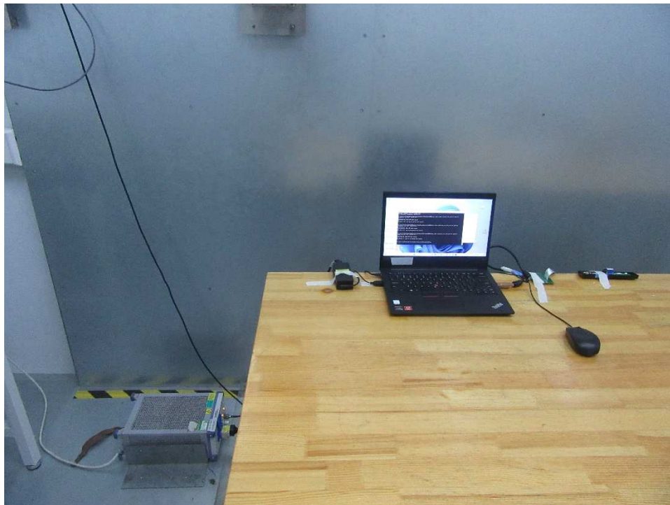
Photograph 9: Set-up for Conducted Emission on AC Mains
