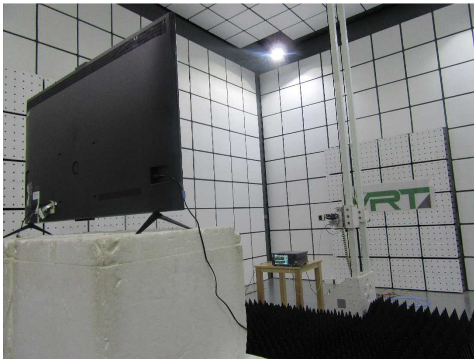
Photograph 12: Set-up photo for Radiated Spurious Emission, 18GHz - 40GHz
