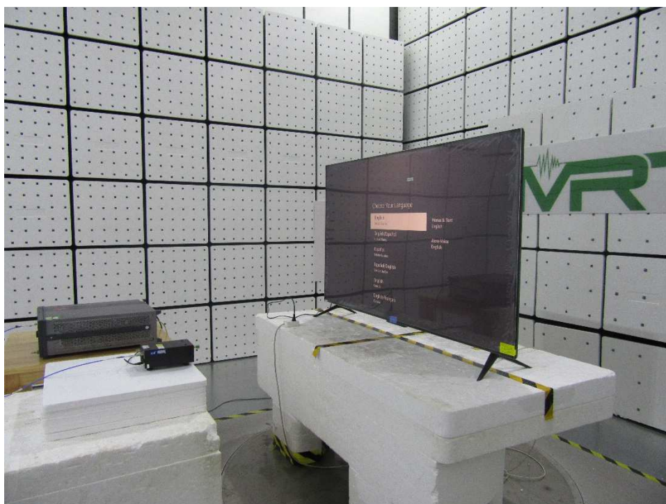
Photograph 17: Set-up photo for Radiated Spurious Emission, 140GHz - 200GHz
