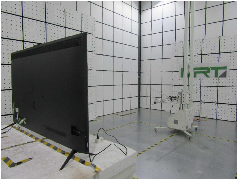
Photograph 10: Set-up photo for Radiated Spurious Emission, below 1GHz
