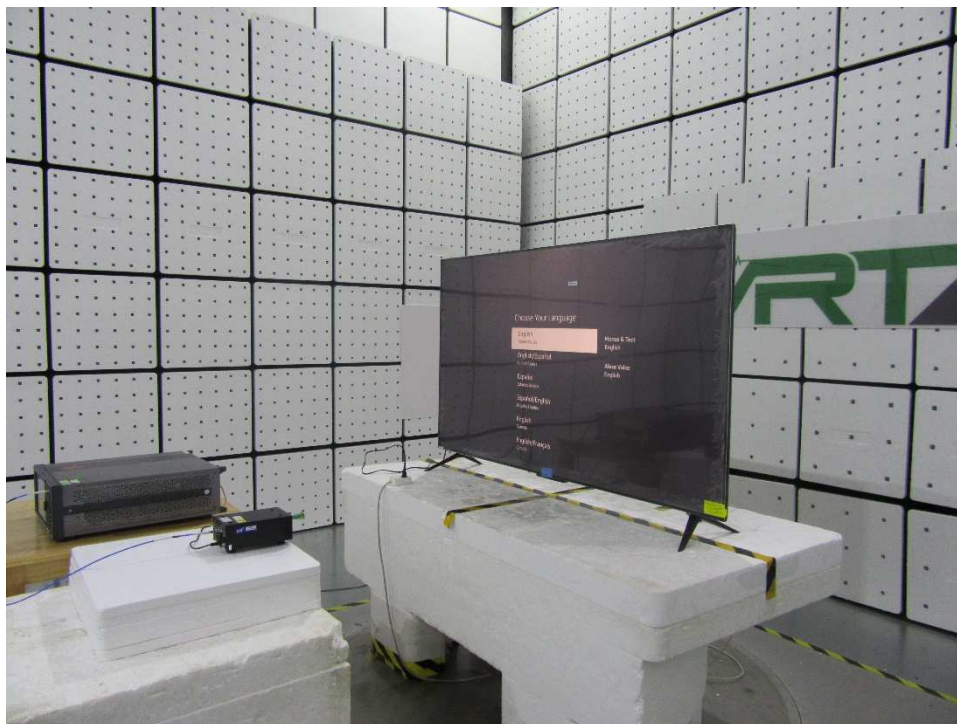
Photograph 16: Set-up photo for Radiated Spurious Emission, 110GHz - 140GHz
