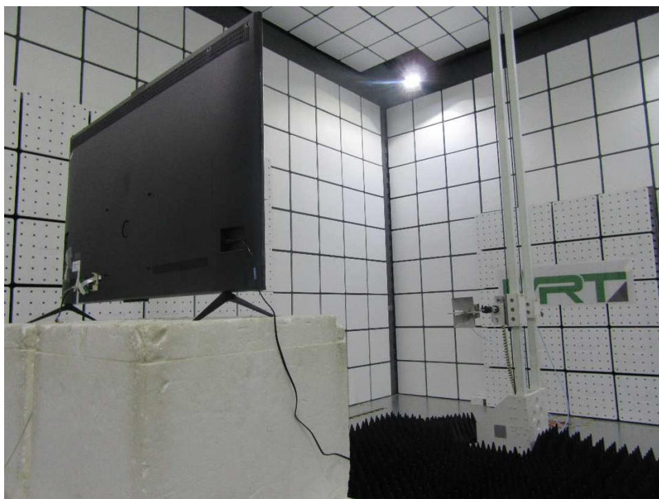
Photograph 11: Set-up photo for Radiated Spurious Emission, 1GHz - 18GHz
