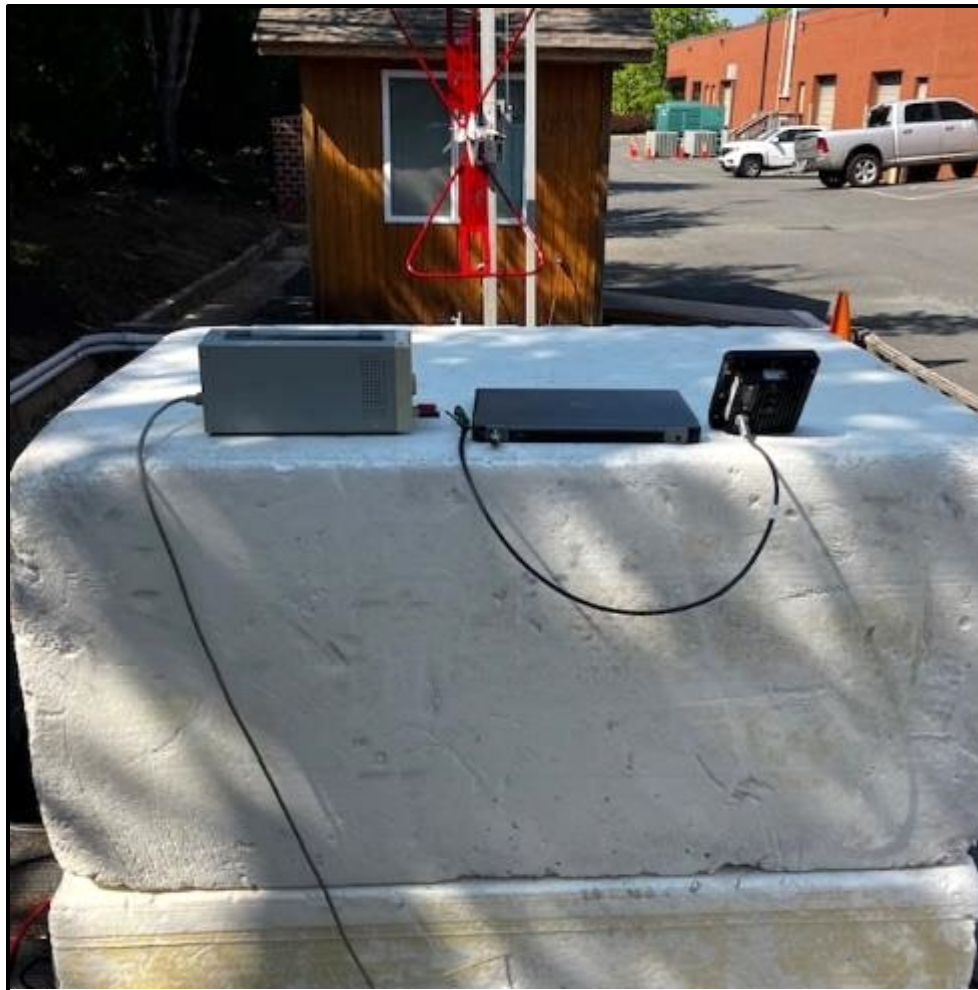
Photograph 4: Radiated Emissions – Back (Greater than 1 GHz)
