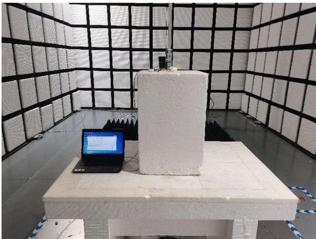
Fig. 3 Radiated emission setup photo(Above 1GHz)
