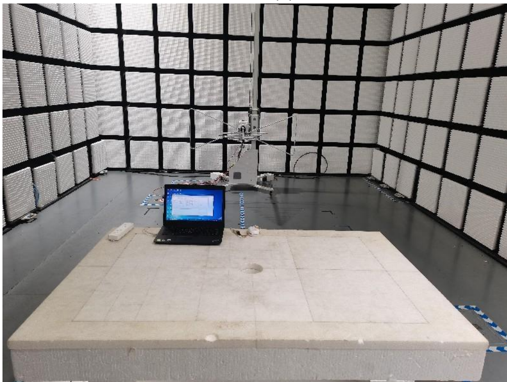
Fig. 2 Radiated emission setup photo(30MHz-1GHz)
