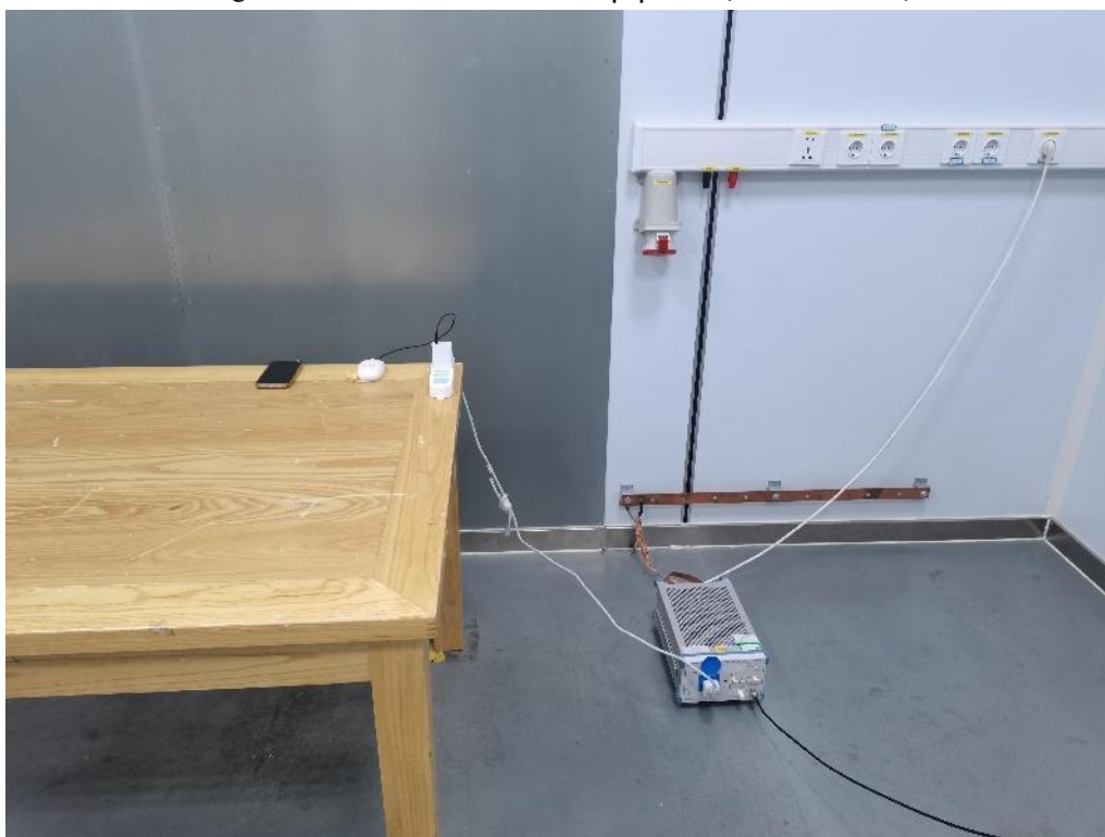
Fig. 4 Power line conducted emission setup photo
