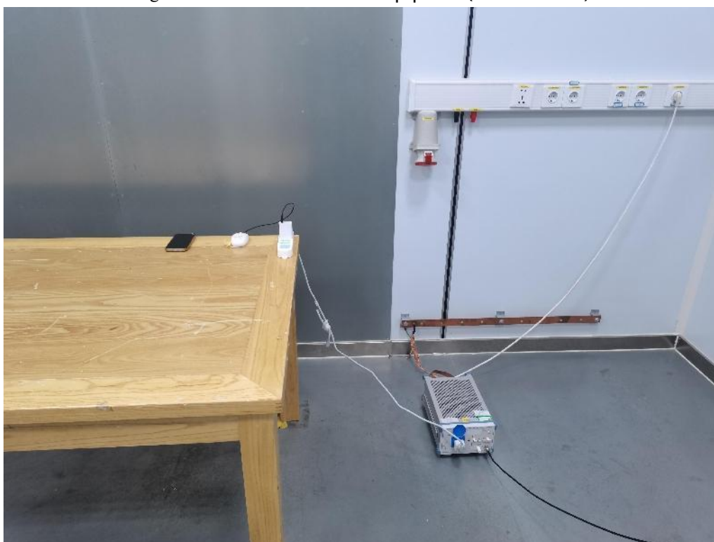
Fig. 4 Power line conducted emission setup photo
