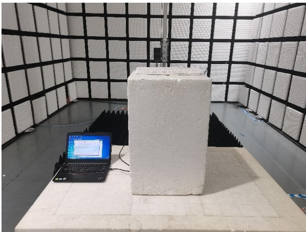
Fig. 3 Radiated emission setup photo(Above 1GHz)
