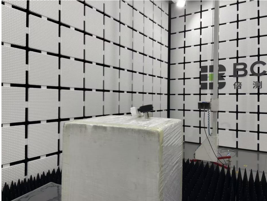
Spurious Emission Test Setup (Above 1GHz)
