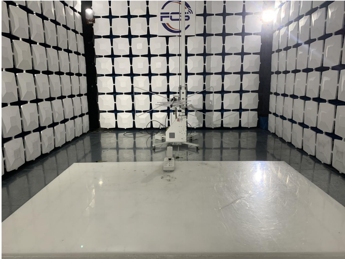
Above 1GHz for radiated emission test setup
