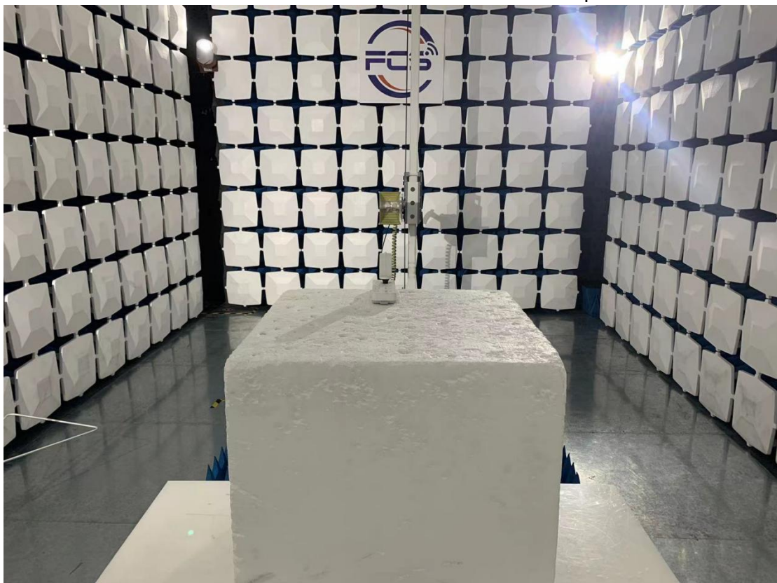
Above 1GHz for radiated emission test setup
