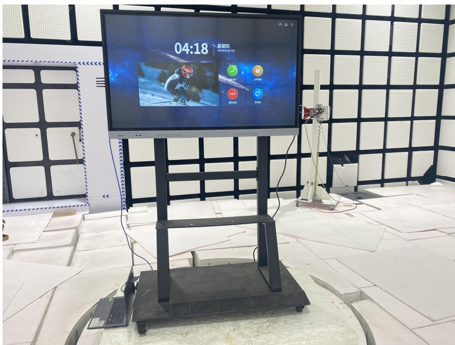
Radiated spurious emission Test Setup-2(Above 1GHz)
