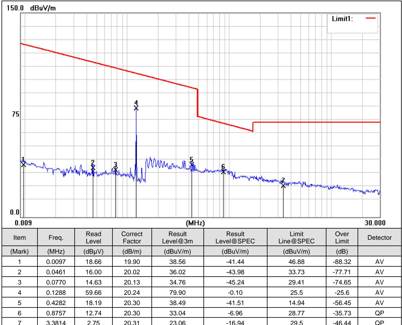
Remark: Result Level= Read Level + Antenna Factor + Cable Loss
