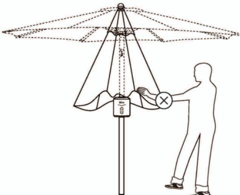
When the motor is working, ensure NO barriers around the surroundings and do NOT move the umbrella or touch components with hands.
