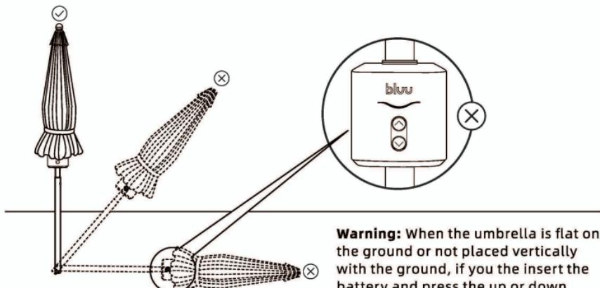
**Warning:** When the umbrella is flat on the ground or not placed vertically with the ground, if you insert the battery and press the up or down button, the motor will stop working and display the red light.
