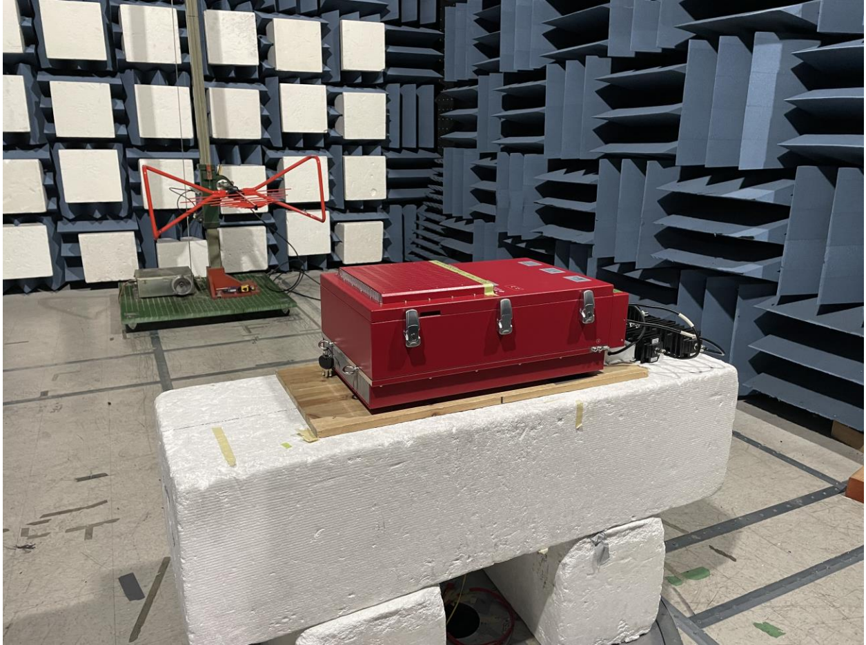
Figure 3: Radiated Emissions Test Setup (30 MHz - 1 GHz)
