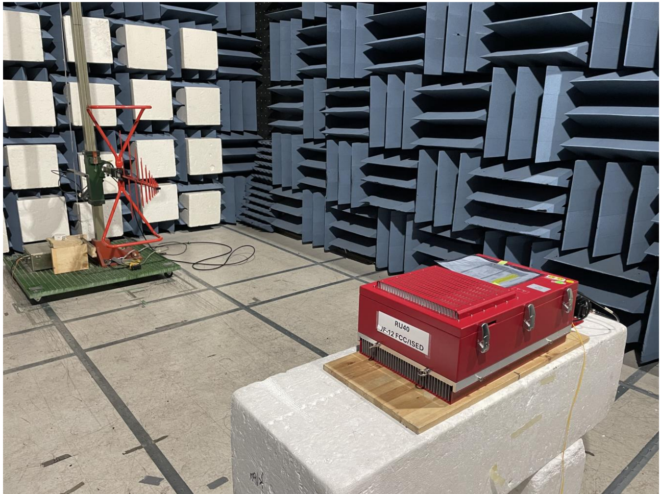
Figure 3: Test setup for radiated emissions between 30 MHz and 1000 MHz
