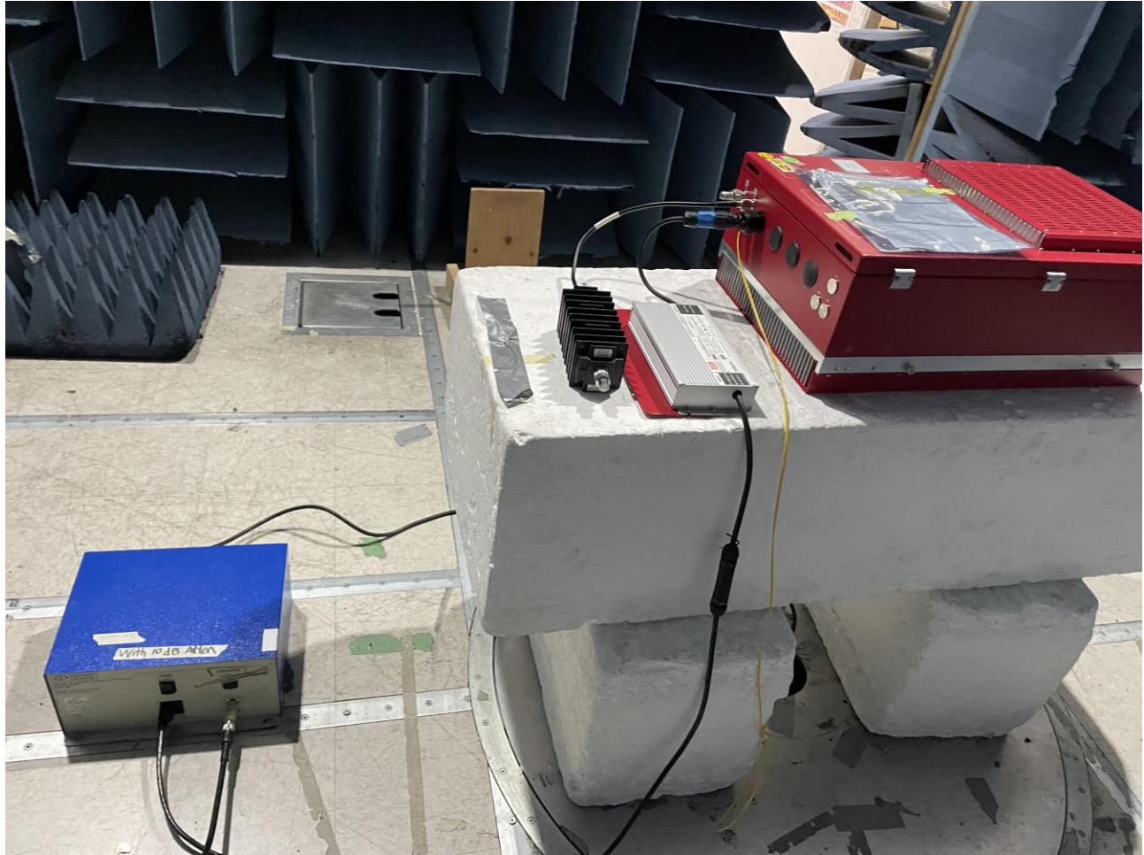
Figure 5: Test setup for conducted emissions
