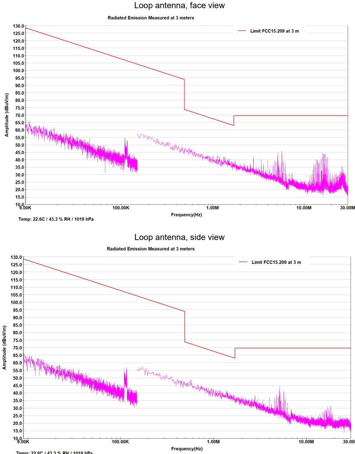
Note (1) No Qpeak measurements were conducted when the emission was identified as either ambient noise or 20 dB, or more, below the limit line.
