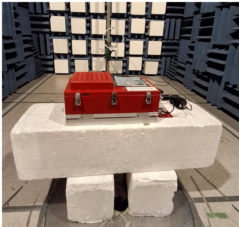
Figure 5: Radiated Emissions Test Setup (Below 30 MHz)
