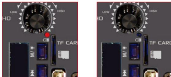
The LED light will turn red while charging and will turn off when the battery is fully charged
