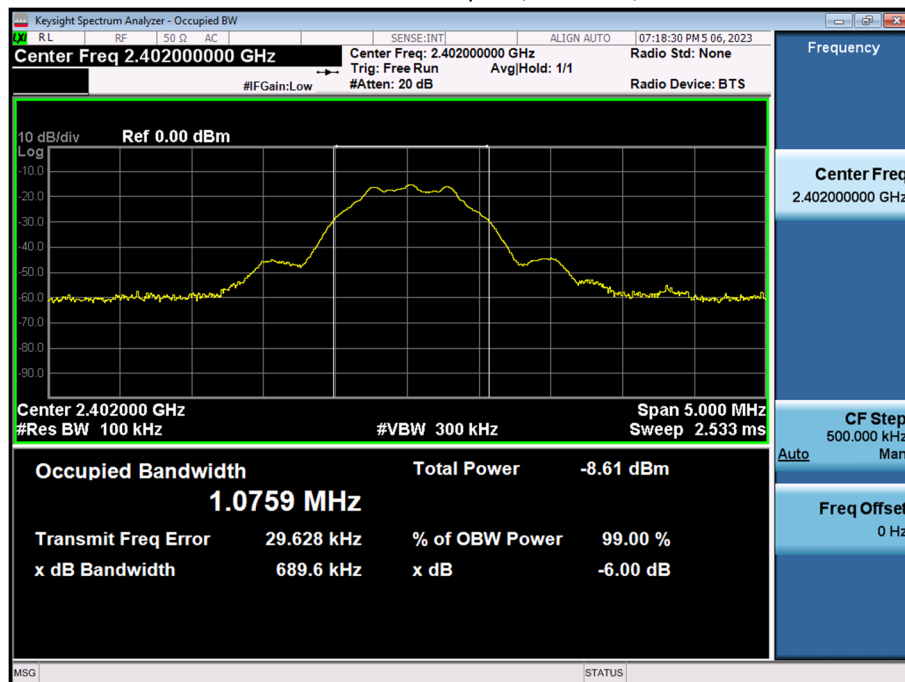
6 dB Bandwidth plot (Low-CH 0)
