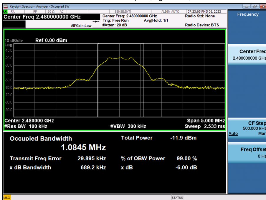
6 dB Bandwidth plot (High-CH 39)
