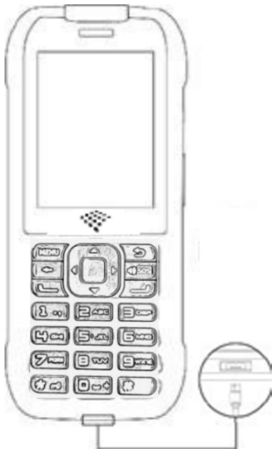
*Note: For first time use, the battery comes partially charged for shipping. It is recommended to charge the battery until full. Use only supplied charger and cable. The use of unauthorized charger carries the risk of damaging the phone or might cause explosion*
