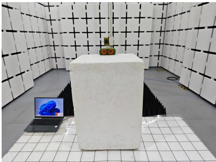
**Conducted Emission Test Setup Photo**
