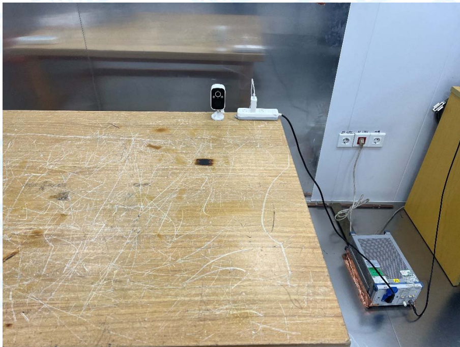
Photo of Setup for Conducted Emission
