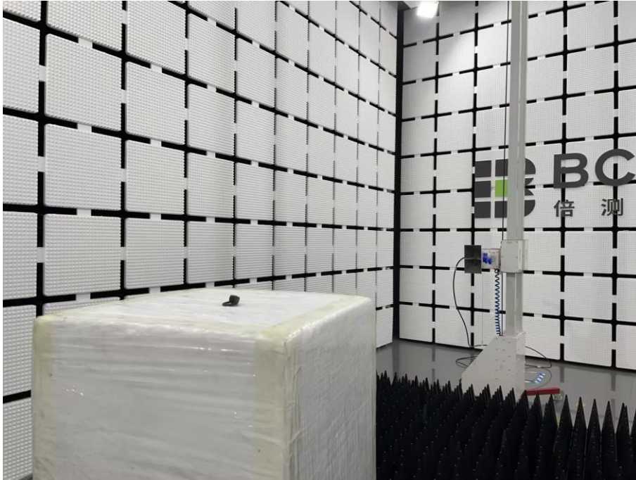
Spurious Emission Test Setup (Above 1GHz)
