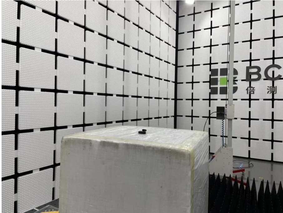
Spurious Emission Test Setup (Above 1GHz)
