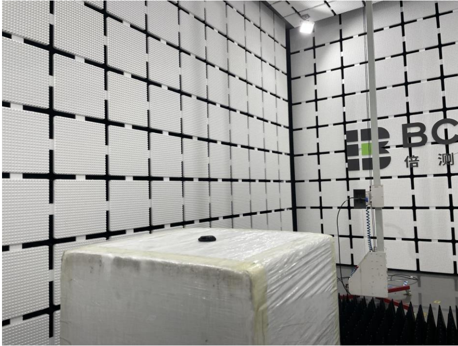
Spurious Emission Test Setup (Above 1GHz)
