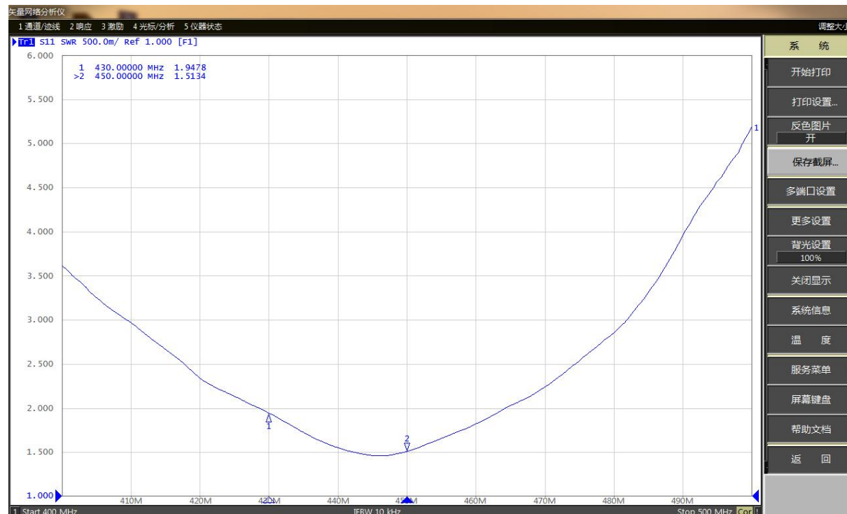
Attachment 1: VSWR Typical Test Figure
