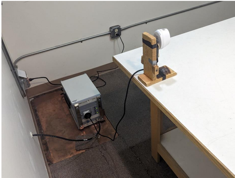
Photograph 8: Back View Conducted Emissions Worst-Case Configuration
