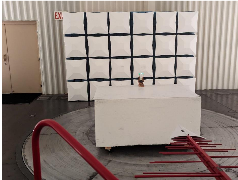
Photograph 3: Front View Radiated Emissions Worst-Case Configuration – Frequencies 30-1000MHz
