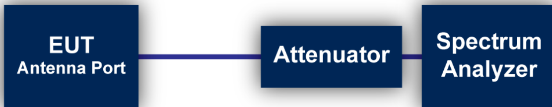
Figure 2: Direct Connection at the Antenna Port Test
