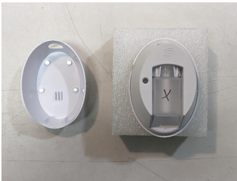
Photograph 10: Front View of the EUT with Cover Removed and Tag In Place
