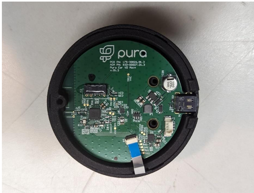
Photograph 14: View of the EUT with Cover and Battery Removed Showing How PCB Fits in Enclosure
