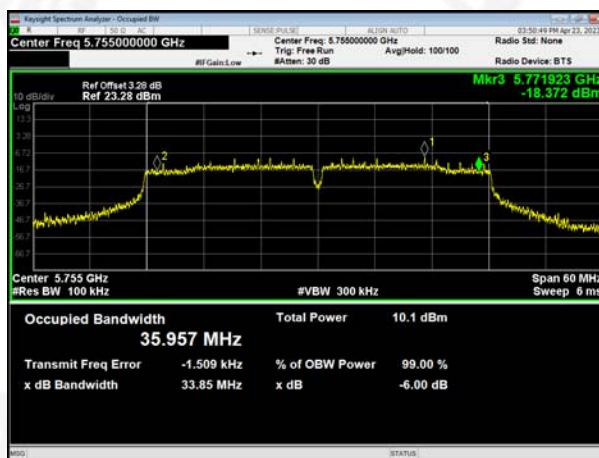
(802.11 ac40) 6dB Bandwidth plot on channel 159
