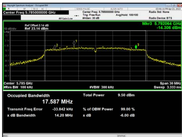
(802.11ac20) 6dB Bandwidth plot on channel 165
