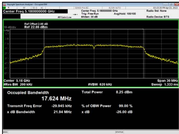
(802.11 n20) 26dB Bandwidth plot on channel 40
