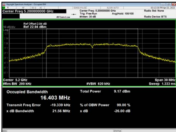
(802.11 a20) 26dB Bandwidth plot on channel 40
