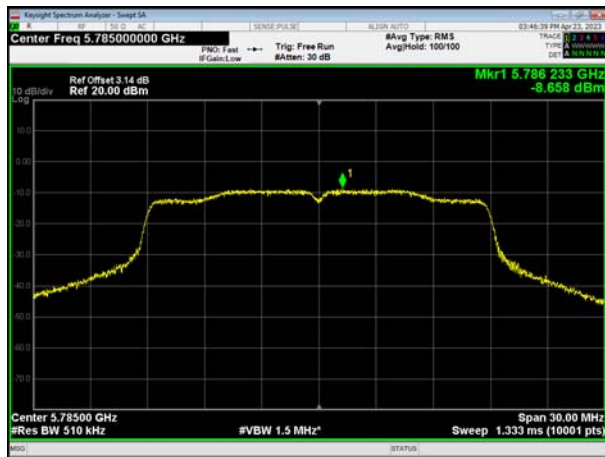
(802.11ac20) PSD plot on channel 165
