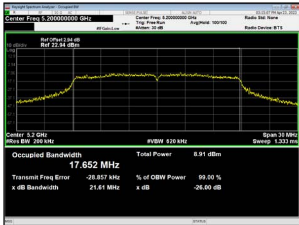
(802.11 n20) 26dB Bandwidth plot on channel 48
