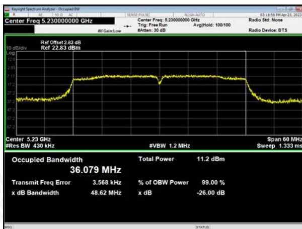
(802.11 ac40) 26dB Bandwidth plot on channel 42
