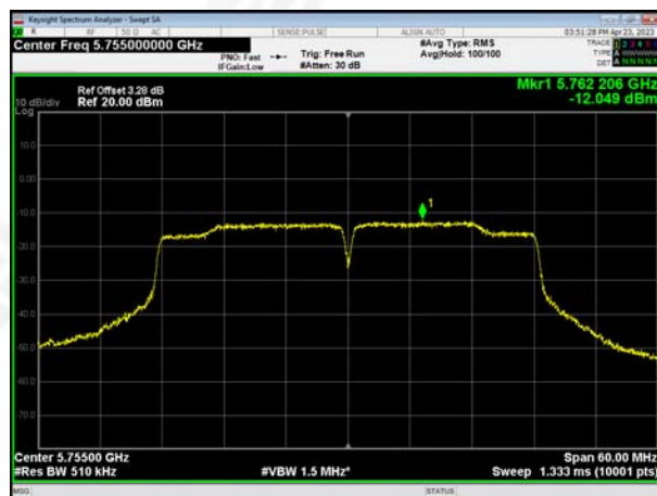
(802.11n40) PSD plot on channel 159
