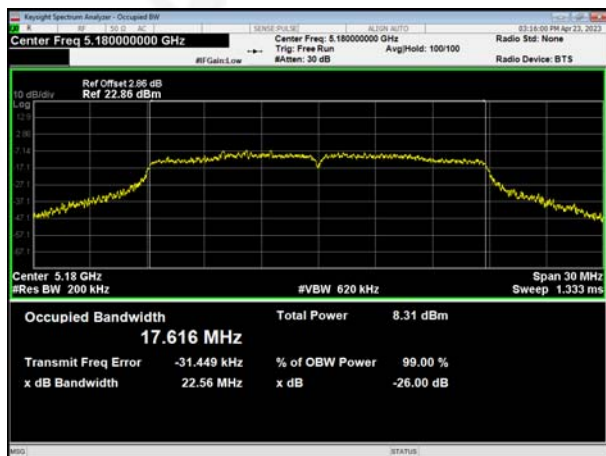
(802.11ac20) 26dB Bandwidth plot on channel 40
