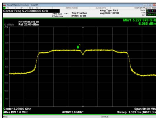
(802.11ac80) PSD plot on channel 42
