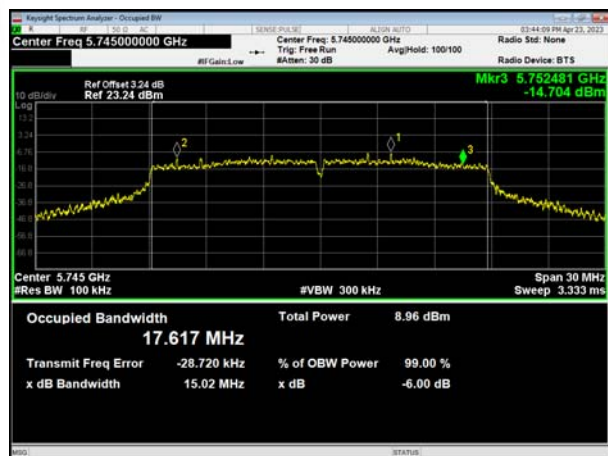
(802.11n20) 6dB Bandwidth plot on channel 149
