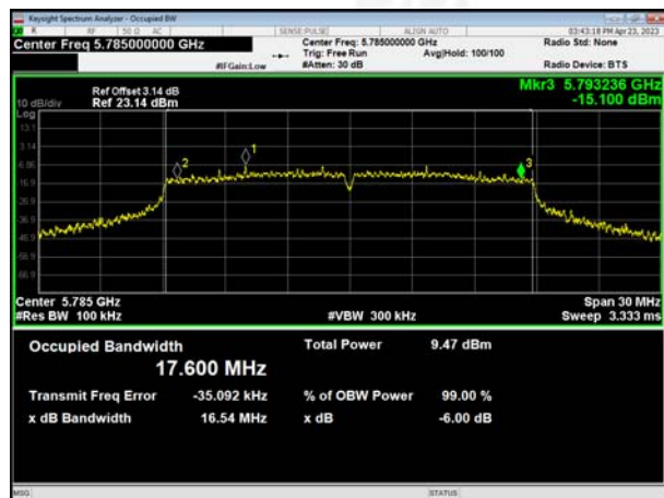
(802.11n20) 6dB Bandwidth plot on channel 165
