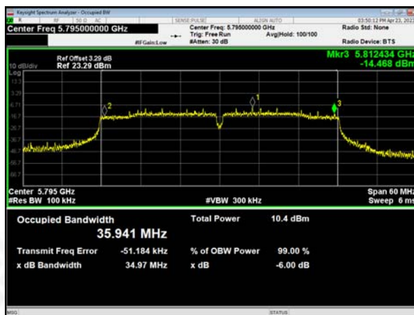
(802.11 ac40) 6dB Bandwidth plot on channel 159
