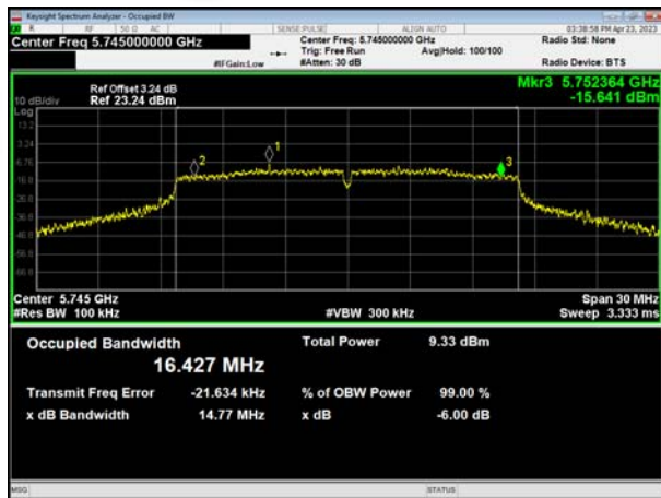
(802.11a20) 6dB Bandwidth plot on channel 149
