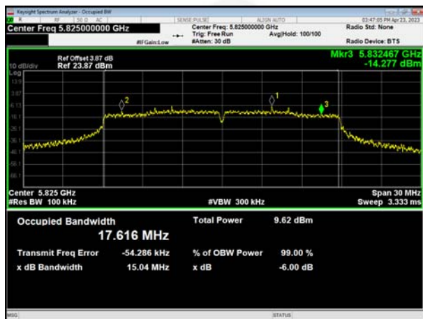
(802.11ac20) 6dB Bandwidth plot on channel 165
