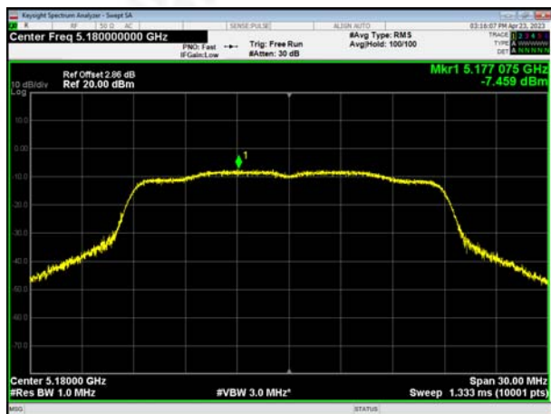
(802.11ac20) PSD plot on channel 40
