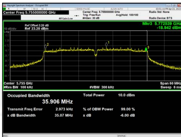
(802.11 n40) 6dB Bandwidth plot on channel 151
