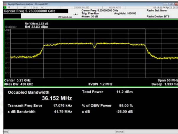
(802.11 n40) 26dB Bandwidth plot on channel 46
