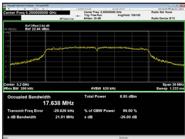
(802.11ac20) 26dB Bandwidth plot on channel 40
