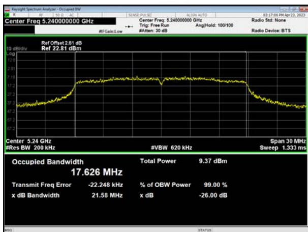
(802.11ac20) 26dB Bandwidth plot on channel 48
