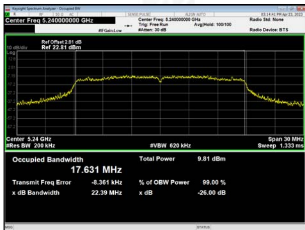
(802.11 n20) 26dB Bandwidth plot on channel 48
