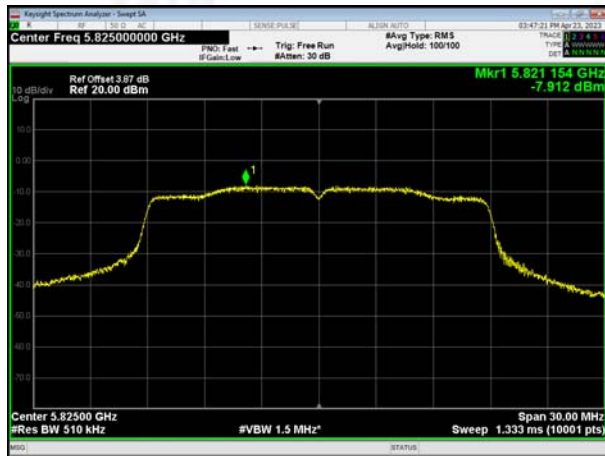
(802.11ac20) PSD plot on channel 165
