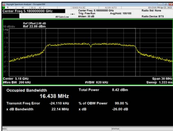
(802.11 a20) 26dB Bandwidth plot on channel 36
