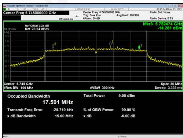
(802.11ac20) 6dB Bandwidth plot on channel 157
