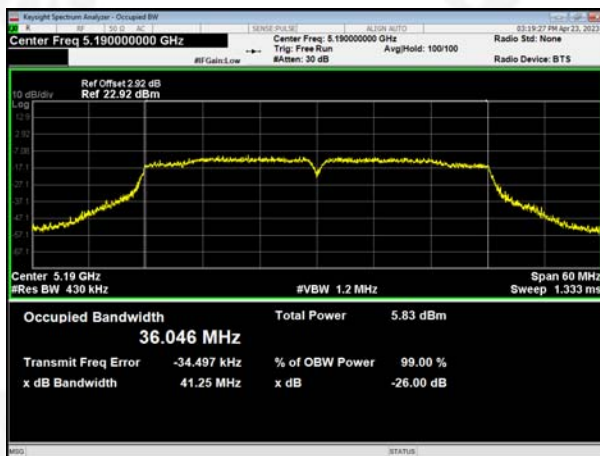
(802.11 ac40) 26dB Bandwidth plot on channel 42
