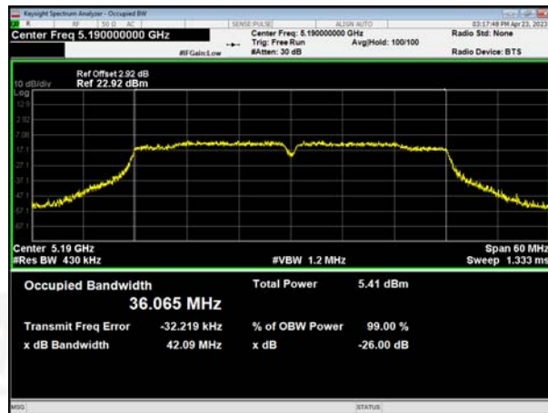
(802.11 n40) 26dB Bandwidth plot on channel 46
