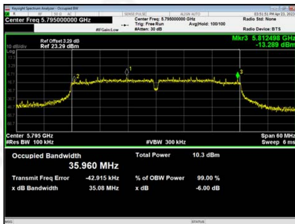
(802.11 n40) 6dB Bandwidth plot on channel 159
