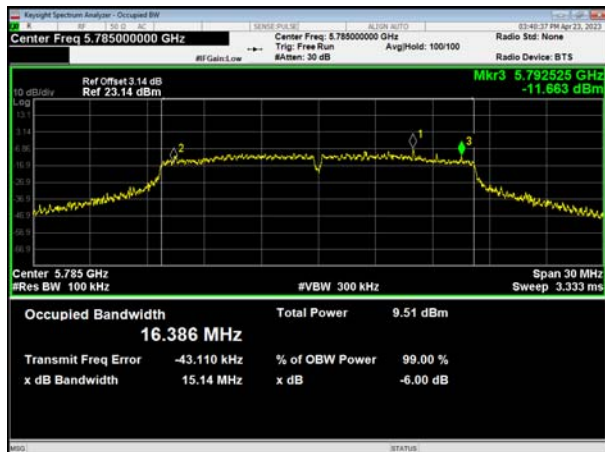
(802.11a20) 6dB Bandwidth plot on channel 157
