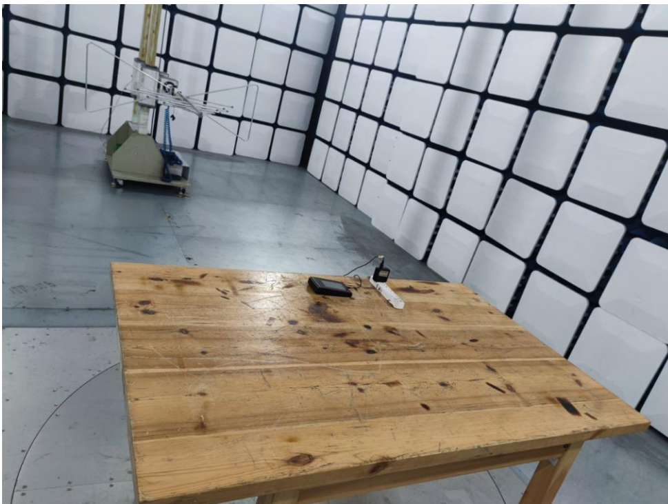
Photo of Radiation Emission Test
