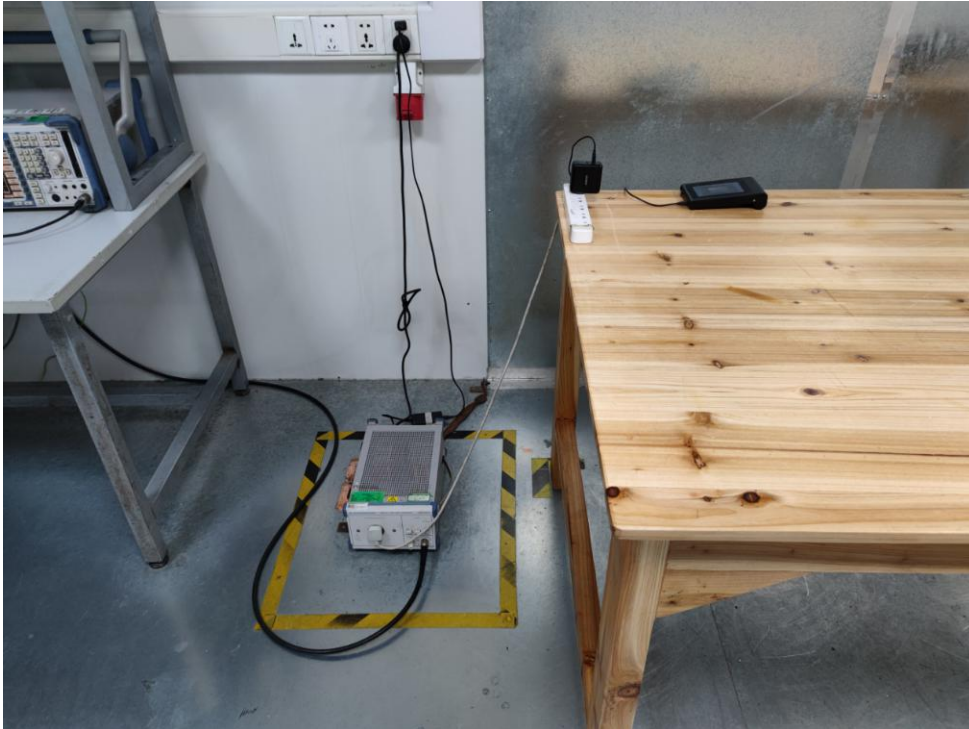
Photo of Power Line Conducted Emission Test
