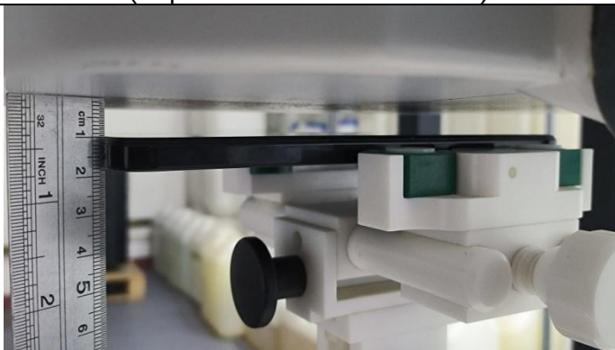
Front Side (Separation distance of 10mm)
