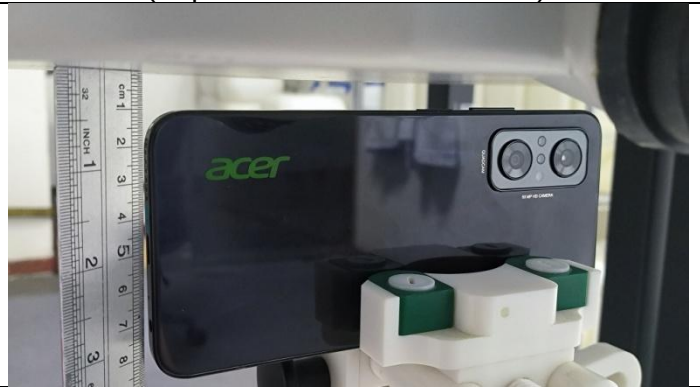
Bottom Side (Separation distance of 10mm)
