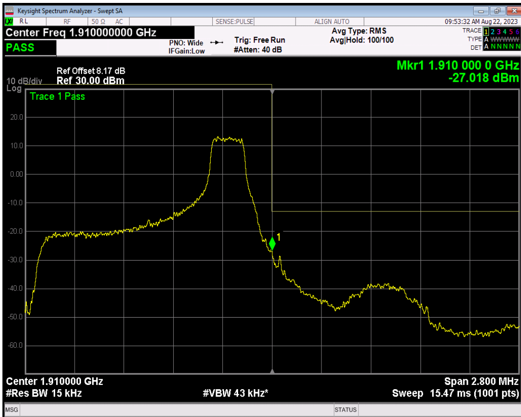
Band2 16QAM BW=1.4MHz Channel=19193 RB Size=6 Position=#0
