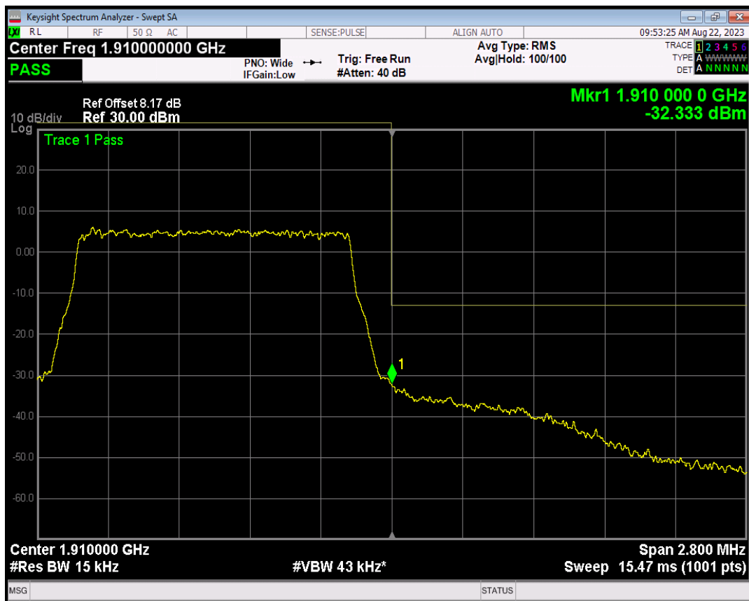
Band2 16QAM BW=1.4MHz Channel=19193 RB Size=1 Position=#0
