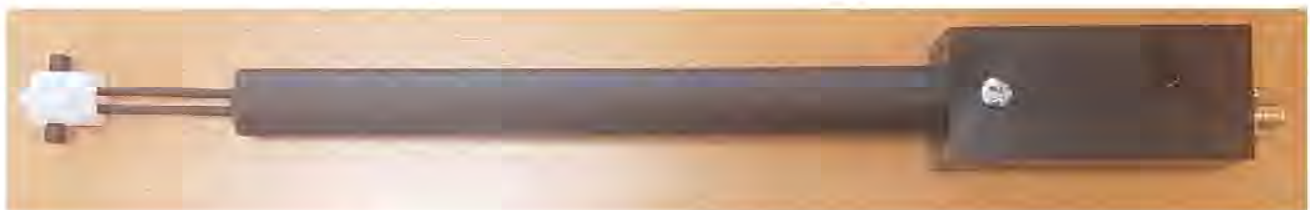
Figure 1 – MVG COMOSAR Validation Dipole
