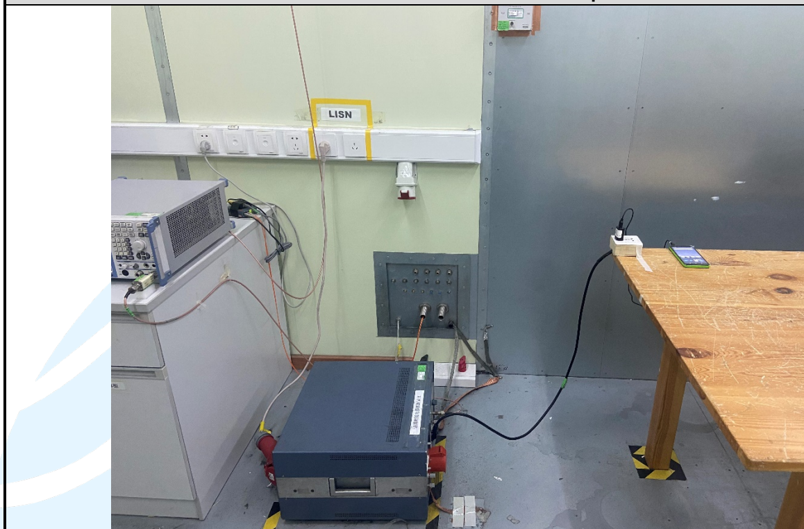
Conducted Emission Test Setup
