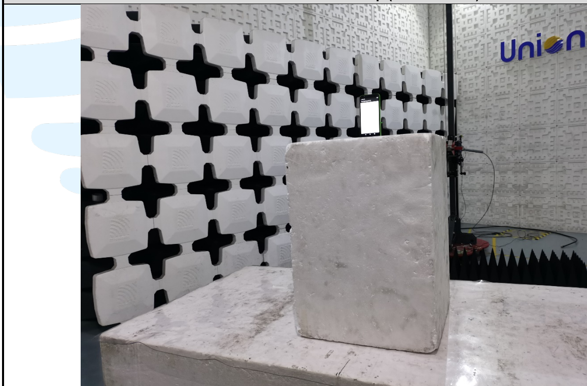
Radiated emission Test Setup (Above 1 GHz)
