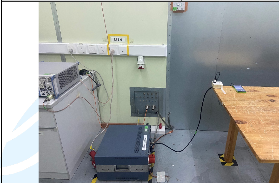
Conducted Emission Test Setup-3 – Test Mode 2
