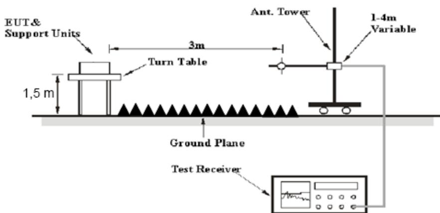
The radiated emission below 1GHz tests were performed in the 10 meters chamber test site, above 1GHz tests were performed in the 3 meters chamber test site B, using the setup accordance with the ANSI C63.10-2013. The specification used was the FCC 15.209, and FCC 15.247 and the RSS-247 Clause 5.5, RSS-GEN Clause 8.10 limits.
